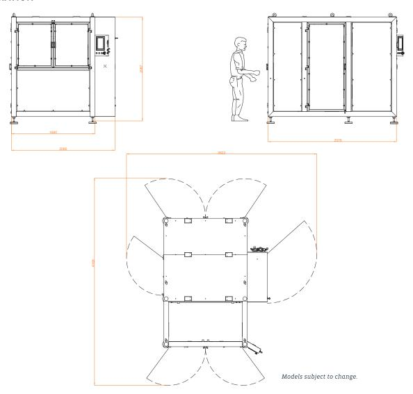
One of the most outstanding features of the INVpack multi-track vertical machines is optimization of production costs with regard to productivity/m2. The INV-Easy design enables safe access to the different areas of the machine, thus facilitating cleaning and maintenance. Possibility of integrating an inline checkweigher.
