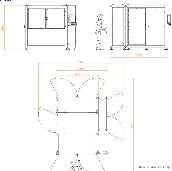
One of the most outstanding features of the INVpack multi-track vertical machines is optimization of production costs with regard to productivity/m2. The INV-Easy design enables safe access to the different areas of the machine, thus facilitating cleaning and maintenance. Possibility of integrating an inline checkweigher.
