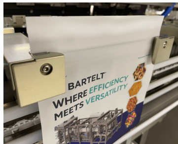
MAGNETIC GRIPPERS Durable and maintenance-free, delivering a strong hold, reduces product buildup, and are easy to clean.
